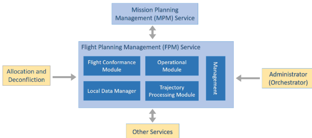
Figure 8 Internal architecture - FPM service
