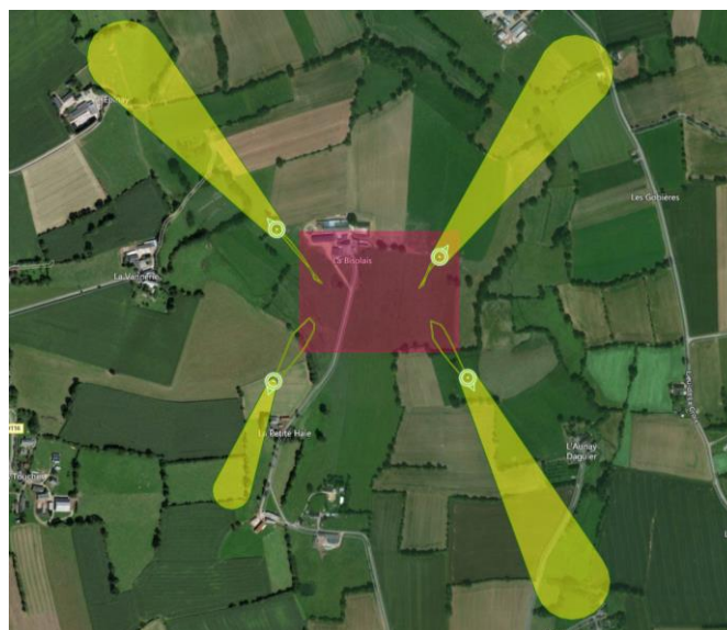
Figure 46: A new flight restriction and all airborne drones within this region exiting the restricted zone
