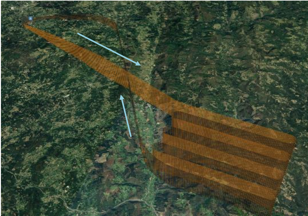
Figure 15. Mission Trajectory for scenario WX-1: East-West surveillance pattern
