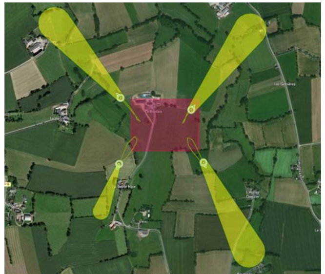
Figure 5. Visualization of a new flight airspace restriction and all airborne drones within this region exiting the restricted zone
